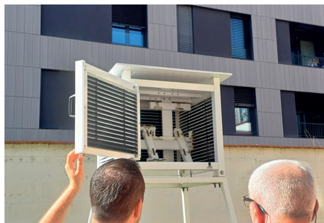
Close-up of the Ecometeo meteorological station and its analogue instruments during installation. (Ecometeo project / Aviation Academy Belgrade)
