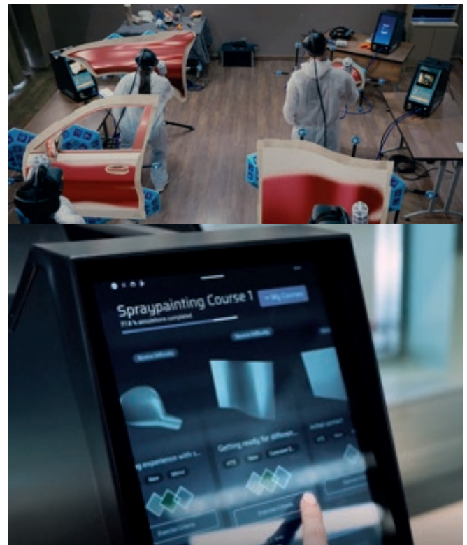
Apprentices are using Seabery Augmented Reality simulators to learn how to paint car parts.
